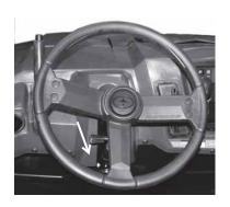
To conserve battery power, the EPS will shut down 5 minutes after the engine is stopped if the key remains in the ON position. The EPS warning indicator will illuminate to indicate the EPS has shut down. Turn the key off and on to reset the unit.
